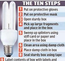
can break if dropped or handled roughly. Always screw and unscrew the lamp by its base and never forcefully twist the CFL into a light socket by its glass tubes.
